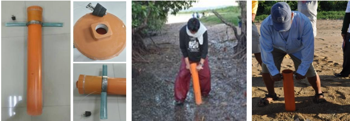
Figure 14. Core sampler constructed from 60cm long PVC Pipe with 10cm diameter; Illustration of sample collection
